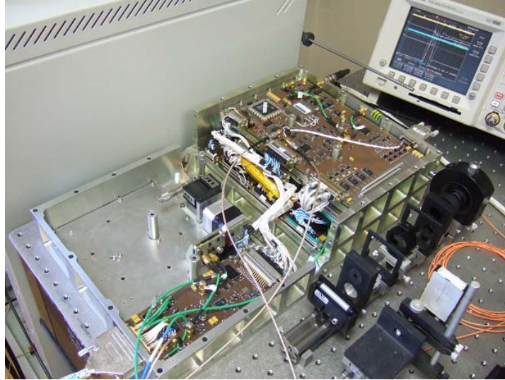
Figure 2. T2L2 engineering model: the electronic Unit, opened, during tests at the OCA.
